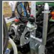
The pump is fitted to the three-point mounting, meaning that no extended PTO shaft is needed, which means the turning radius is very narrow.
