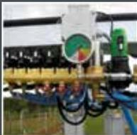
Valve unit for six boom sections, with electric pressure adjustment.
