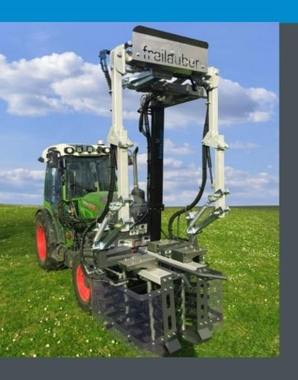
In order to protect the device, all four roll holders come with a collision protection system. The roll holders are held in position by springs so that they can be pressed to the outside by bended sticks to avoid damage both at trunk as well as device.
