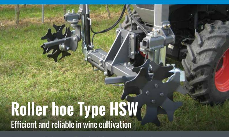
The Type HSW roller hoe is used for herbicide-free control of weeds in the vine row. It loosens the ground along the vine row in a strip of about 120 to 180mm long (depending on the working angle that was set and the discs' undercut) and as it does so buries weeds with the loosened earth.
